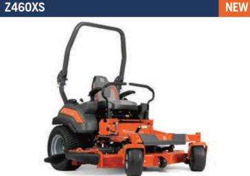
Each model in Husqvarna's Z400 Series of zero-turn mowers boasts an optimal weight balance that holds hills and maintains traction. The Parker HTE Series transmission delivers more power, quieter performance, 10% better fuel efficiency and an operating temperature that's as much as 50°F cooler.
